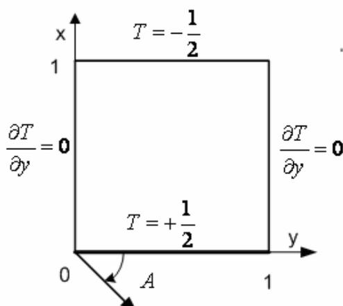
Figure 1. Thermal conditions on the cavity walls. The gravity direction shown by the arrow forms angle  $A$  with the  $y$  axis.
