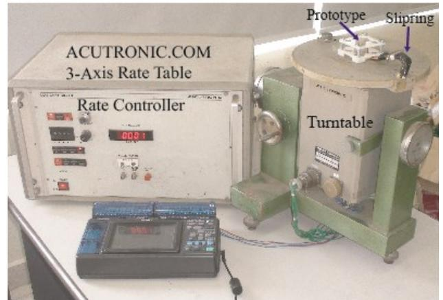
Figure 5: The fabricated prototype is mounted on a standard Acutronic turntable.
