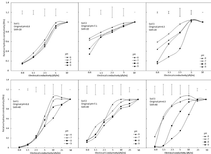
Figure 1 Effects of wastewater pH 6, 7, 8 and 9 on hydraulic conductivity at different electrical conductivity for soils at SAR=20 and 40. Bars represent HSD values for each event.
