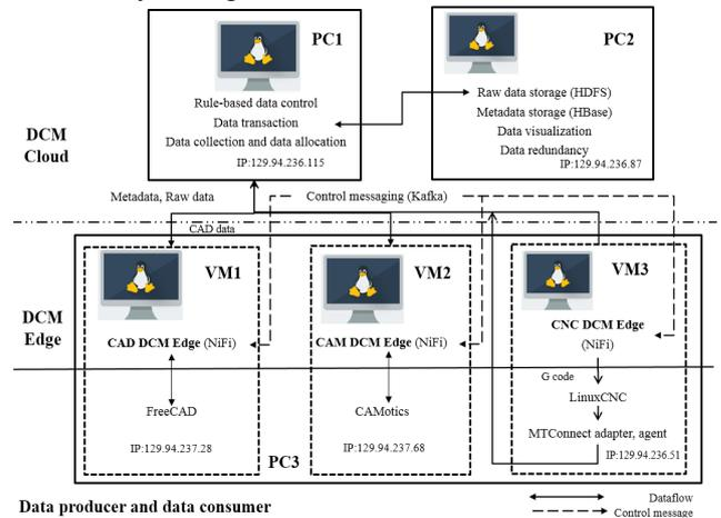
Fig. 3. The experiment setup of the designed system
