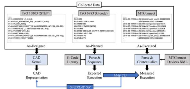
Fig. 1. Overview of technical approach to link as-planned to as-executed data and overlay results on CAD representation [3]
