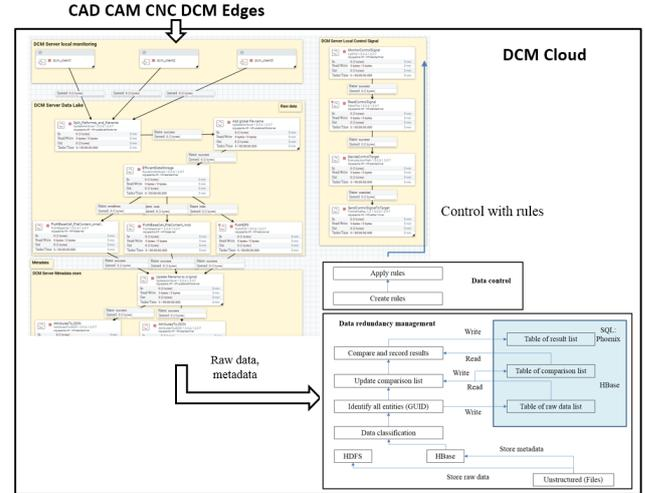
Fig. 5. The flowchart of the developed DCM Cloud
