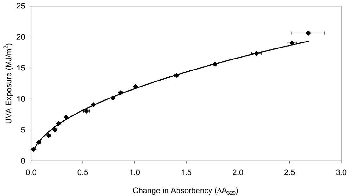
**Figure 4.** Calibration curve of PPO for solar UVA exposures. The error bars represent the standard deviation in each series of absorbency measurements.
