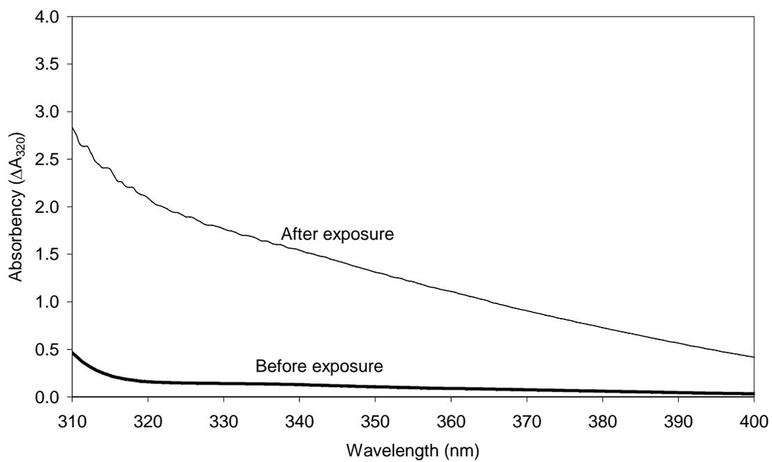
**Figure 3.** The absorption spectrum of PPO before and after a total solar UVA exposure of  $20 \text{ MJ/m}^2$ .
