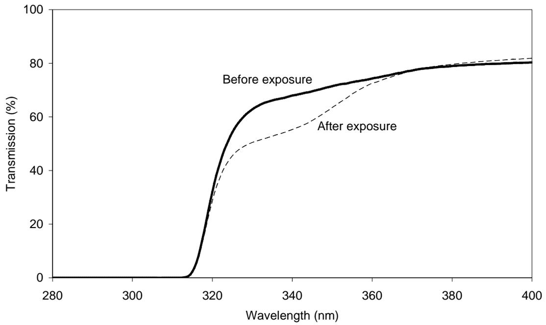
**Figure 2.** The spectral transmission of mylar film before and after a total solar UVA exposure of  $20 \text{ MJ/m}^2$ .
