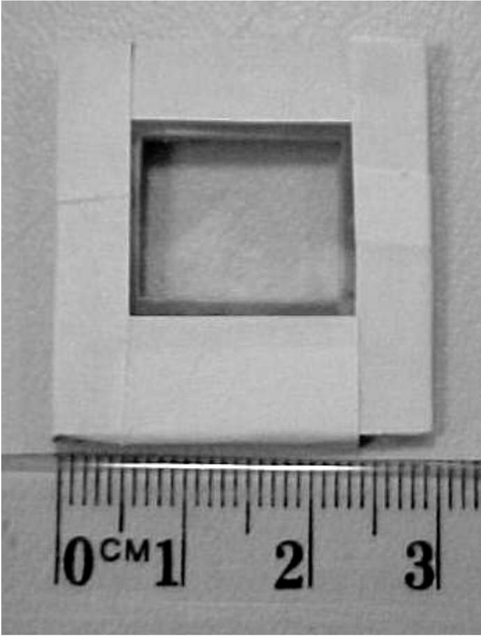
**Figure 1.** A sample PPO dosimeter with the mylar film attachment.
