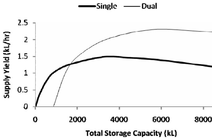
**Figure 7:** Base scenario storage capacity-supply yield curves for Single Storage and Dual Storage systems
