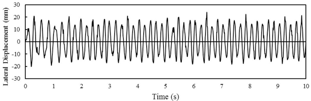
Fig. 3. The top lateral displacements of bare specimens
