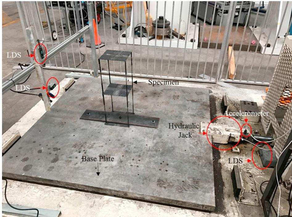
Fig. 2. Experimental set-up
