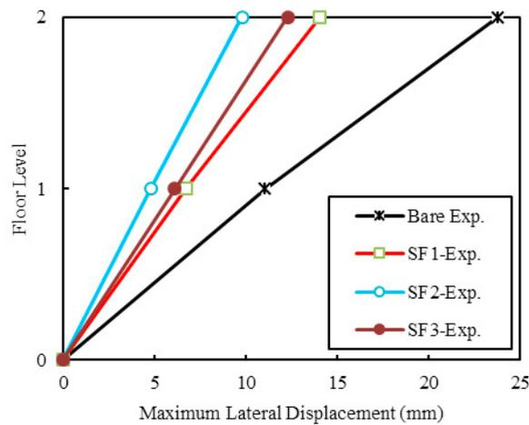
Fig. 7. Comparison of maximum lateral displacements at each floor level
