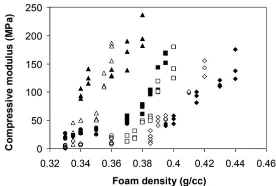
**Figure 2** (a) Compressive modulus as function of foam density:  $\blacktriangle$ , SL75 pre-mould gelatinisation;  $\triangle$ , SL75 post-mould gel;  $\blacksquare$ , SL150 pre-mould gel;  $\square$ , SL150 post-mould gel;  $\blacklozenge$ , SL300 pre-mould gel;  $\diamond$ , SL300 post-mould gel;  $\bullet$ , SL500 pre-mould gel; and  $\circ$ , SL500 post-mould gel.
