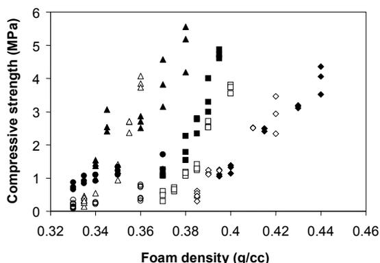
**Figure 1** Compressive strength vs foam density: ▲, SL75 pre-mould gel; △, SL75 post-mould gel; ■, SL150 pre-mould gel; □, SL150 post-mould gel; ◆, SL300 pre-mould gel; ◇, SL300 post-mould gel; ●, SL500 pre-mould gel; and ○, SL500 post-mould gel.
