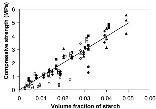
**Figure 3** Compressive strength as function of volume fraction of starch in foam:  $\blacktriangle$ , SL75 pre-mould gelatinisation;  $\triangle$ , SL75 post-mould gel;  $\blacksquare$ , SL150 pre-mould gel;  $\square$ , SL150 post-mould gel;  $\blacklozenge$ , SL300 pre-mould gel;  $\diamond$ , SL300 post-mould gel;  $\bullet$ , SL500 pre-mould gel; and  $\circ$ , SL500 post-mould gel. The least square line is for SL75, SL150 and SL300 collectively.
