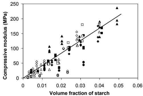
**Figure 4** Compressive modulus vs volume fraction of starch in foam: ▲, SL75 pre-mould gel; △, SL75 post-mould gel; ■, SL150 pre-mould gel; □, SL150 post-mould gel; ◆, SL300 pre-mould gel; ◇, SL300 post-mould gel; ●, SL500 pre-mould gel; and ○, SL500 post-mould gel. The least square line is for SL75, SL150 and SL300 collectively.
