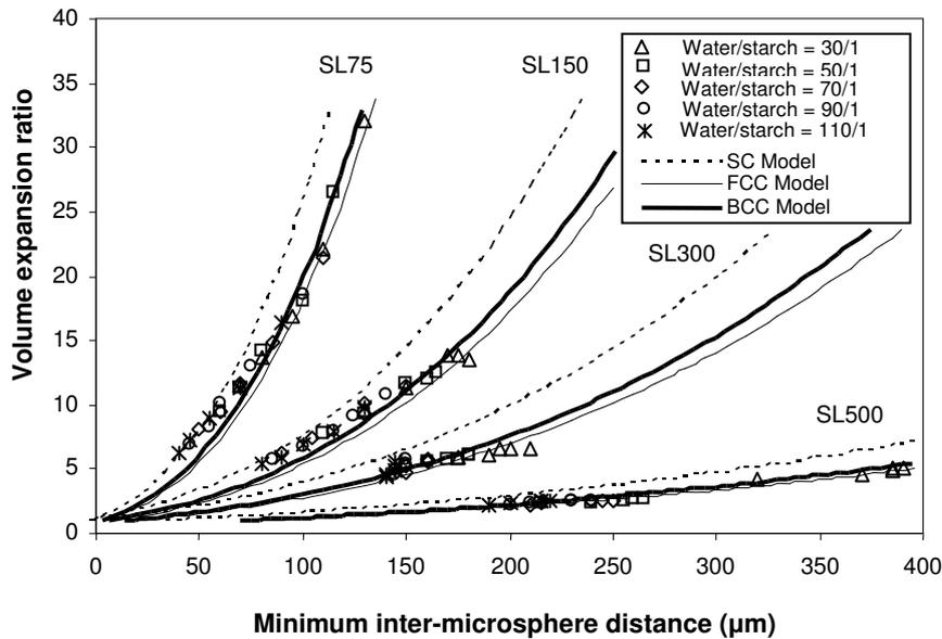
**Figure 1** Experimental volume expansion ratio (VER) versus numerically calculated minimum inter-microsphere distances ( $MID = d_0 + d_e$ ) in comparison with theoretical curves generated according to Eq. 2. The initial bulk volumes of microspheres (10cc, 15cc, 20cc, 25cc and 30cc) for each water/starch ratio are seen such that the higher VER the lower IBVMS.
