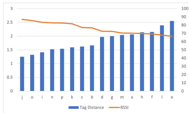
**Figure 5.** Fall in RSSI with tag distance.
