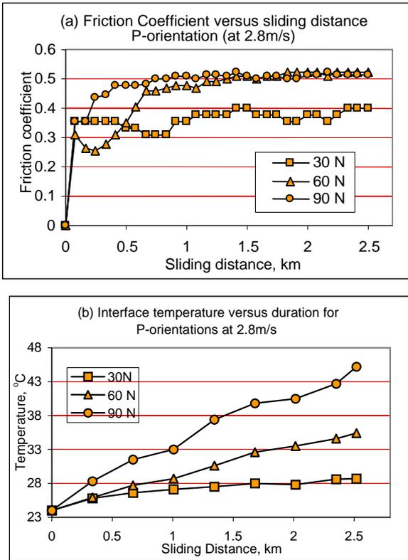
**Fig. 3-** Friction coefficient and interface temperature of CGRP sliding Vs sliding distance showing the effect of applied load in P-orientation at 2.8 m/s
