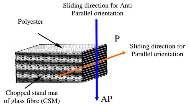
**Fig. 1-** Schematic illustration of CGRP specimens showing the orientations with respect to sliding direction
