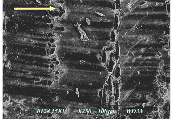
**Fig. 10** SEM photographs of worn surface of CGRP in AP-orientation at 3.9m/s for 2.5 km
