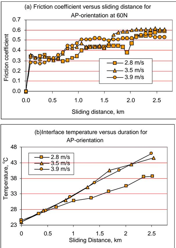
**Fig. 9-** Friction coefficient and interface temperature of CGRP sliding Vs sliding distance showing the effect of sliding velocity AP-orientation at 60N applied load
