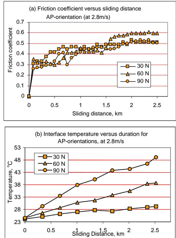
**Fig. 5-** Friction coefficient and interface temperature of CGRP sliding Vs sliding distance showing the effect of applied load in AP-orientation at 2.8 m/s
