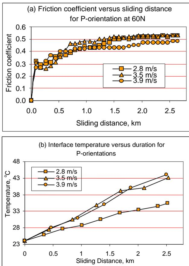
**Fig. 7-** Friction coefficient and interface temperature of CGRP sliding Vs sliding distance showing the effect of sliding velocity P-orientation at 60N applied load
