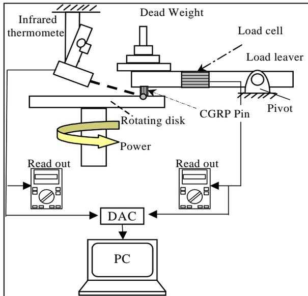
**Fig. 2-** Layout of the experimental set-up for measuring the friction and interface temperature
