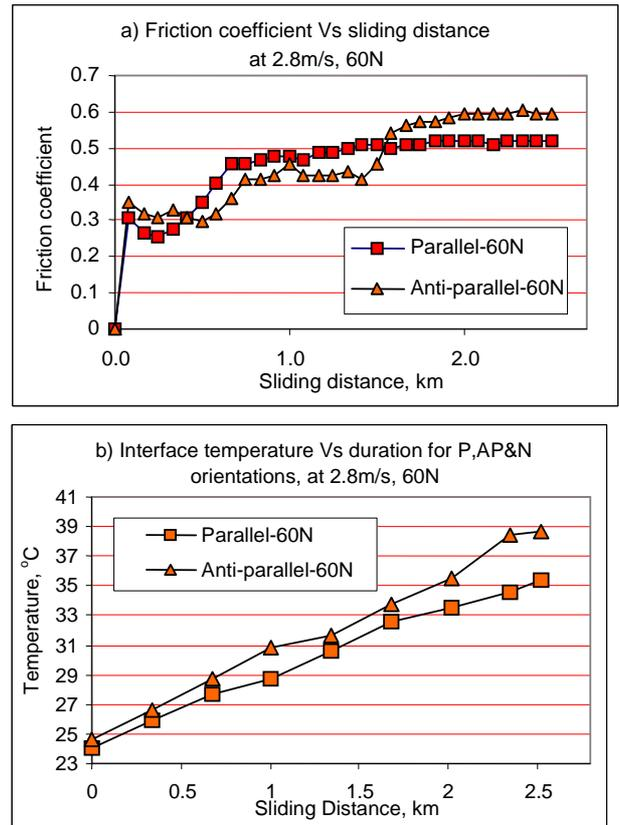
**Fig. 11** Friction coefficient and interface temperature of CGRP at 2.8m/s sliding velocity and 60N applied load for both P and AP-orientations
