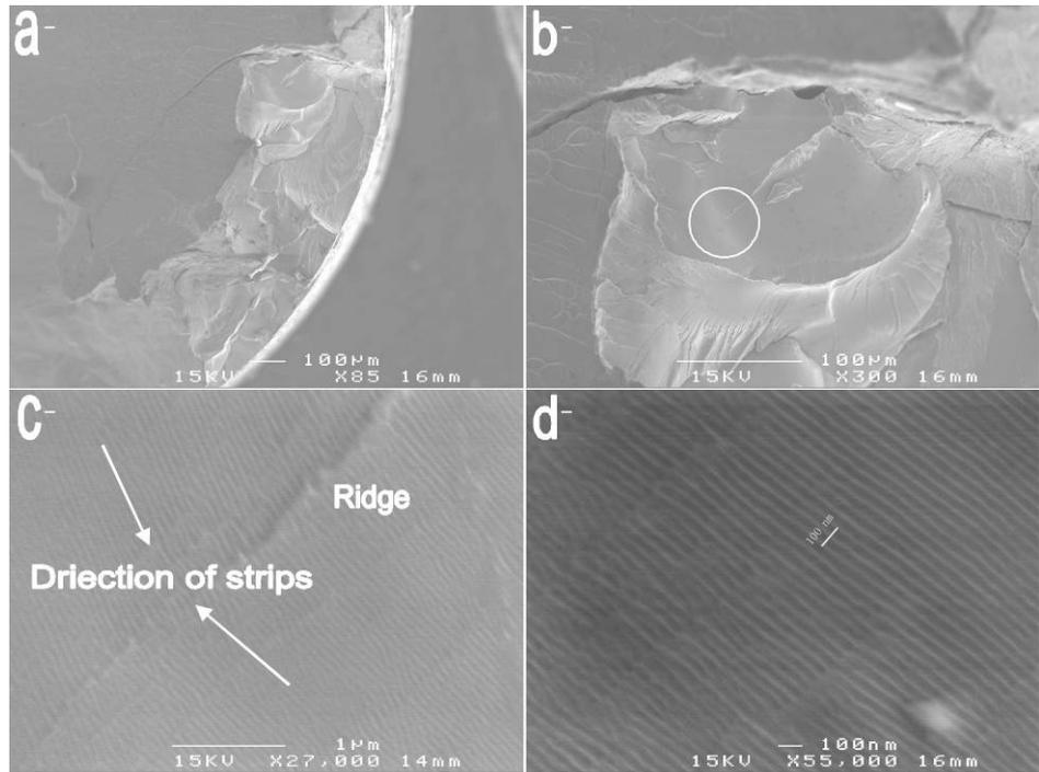
Fig. 1 Macro- (a,b) and micro- (c,d) fracture surface of  $\text{Cu}_{46}\text{Zr}_{45}\text{Al}_7\text{Gd}_2$  alloy
