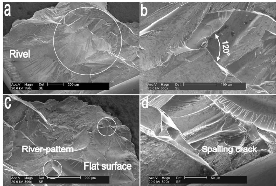
Fig. 2 Macro-fracture surface of  $\text{Cu}_{45.5}\text{Zr}_{45}\text{Al}_7\text{Gd}_{0.5}\text{Ag}_{0.5}$  alloy
