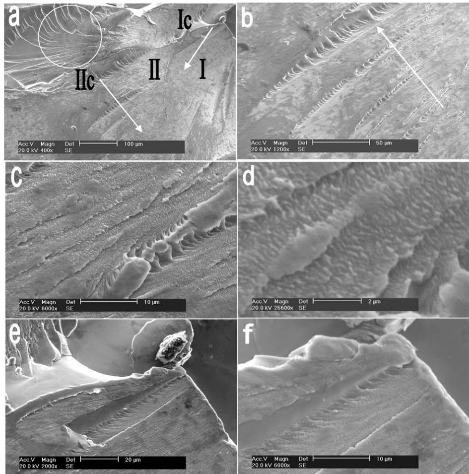
Fig. 3 Micro-fracture surface of  $\text{Cu}_{45.5}\text{Zr}_{45}\text{Al}_7\text{Gd}_7\text{Ag}_{0.5}$  alloy
