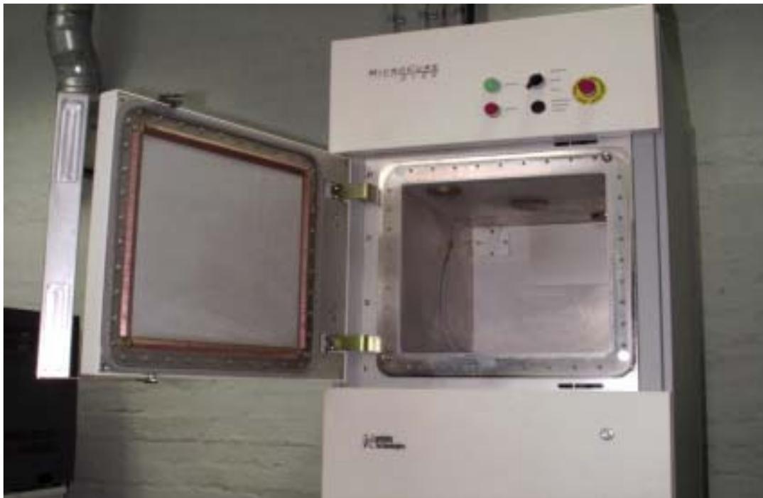
Figure 10: Cavity of Microcure 2100 model 250
