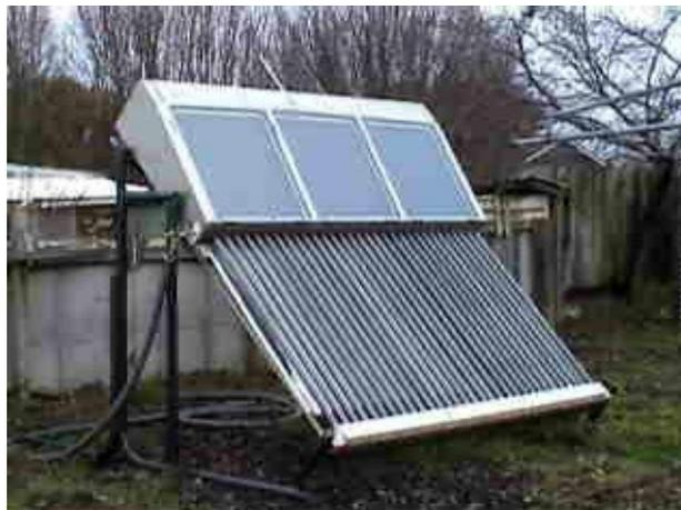
**Figure 1. Evacuated-tubes-flat-plate-combined solar collector, testing prototype.**
