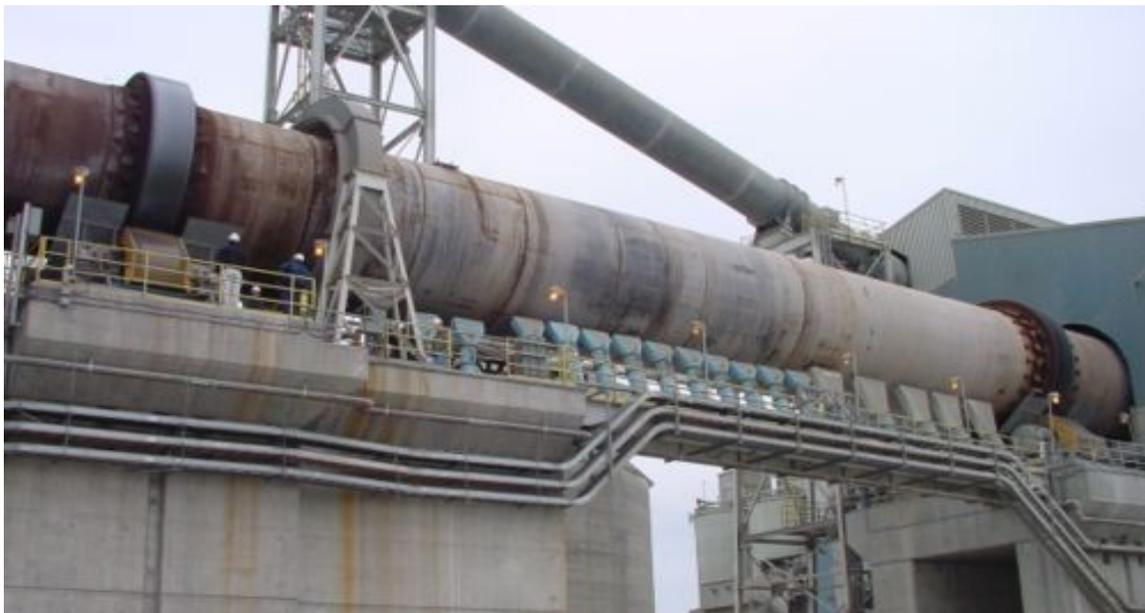
**Figure 3.4: Hot end of medium sized modern cement kiln, showing tyres, rollers and drive gear**
