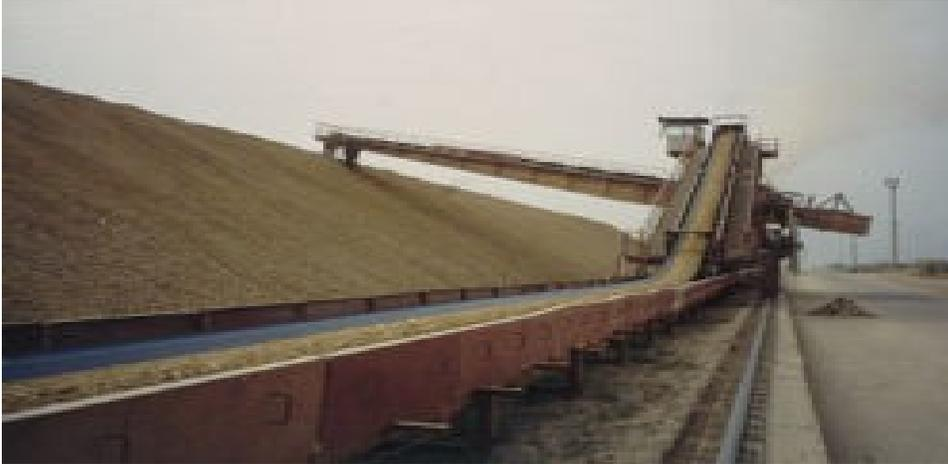
**Figure 3.1: Limestone pre-homogenisation pile being built by a boom stacker**
