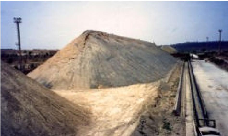
**Figure 3.2: A completed limestone pre-homogenisation pile**
