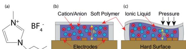
Fig. 1 (a) Chemical structure of [BMIM]<sup>+</sup>[BF<sub>4</sub>]<sup>-</sup>, (b) sensor at rest, (c) sensor under external applied pressure.
