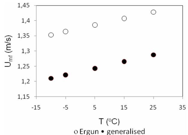
Figure 3. Calculated fluidization behavior
