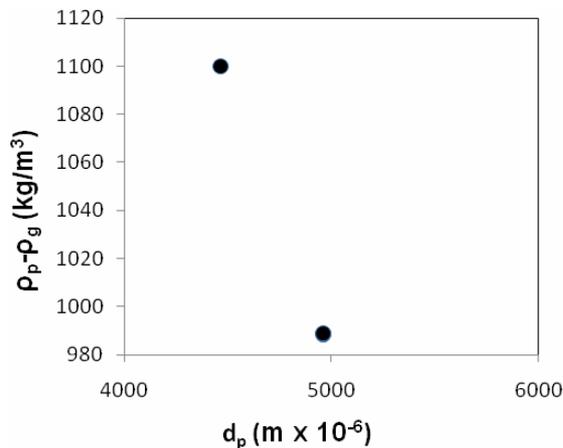
Figure 2. Particle class in Geldart chart
