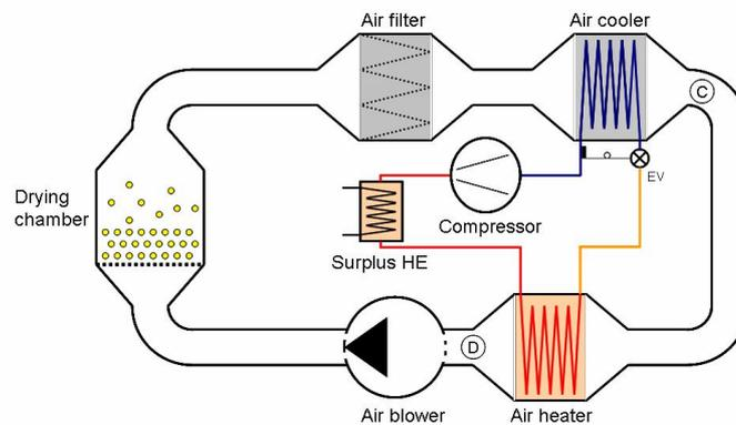
Figure 1. The lay-out of the green heat pump dryer with fluidization
