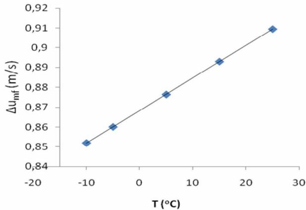
Figure 4. Fluidization velocity versus temperature
