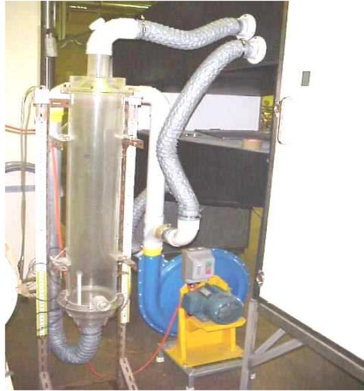
Figure 1 Fluidisation column connected to the heat pump dryer
