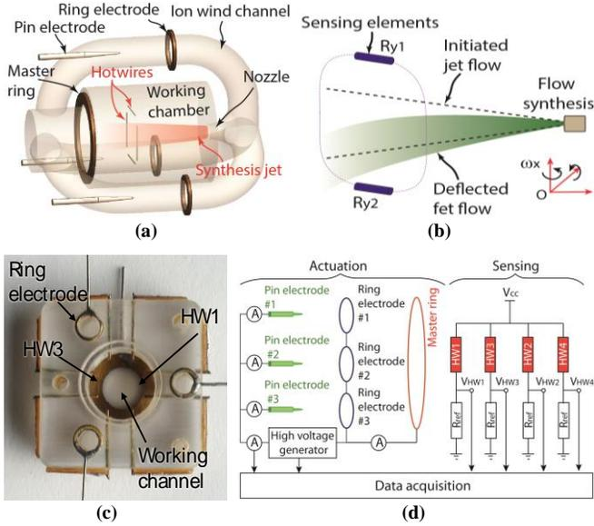
Fig. 1. Mechanism of a jet flow based gyroscope. (a) Hotwire arrangement is to detect the jet flow deflection under the rotations about  $x$ - and  $y$ -axis; (b) Deflection of generated jet flow by the effect of angular velocity; (c) an experimental prototype of the sensor; and (d) measurement circuit.
