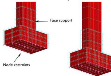
Figure 2 Pier node restraints and face support
