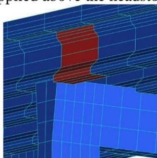
Figure 3 Weakened girder applied above headstock with 3 layers in depth
