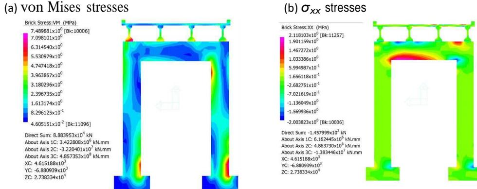
Figure 4 Undamaged bridge stresses under ultimate debris load
