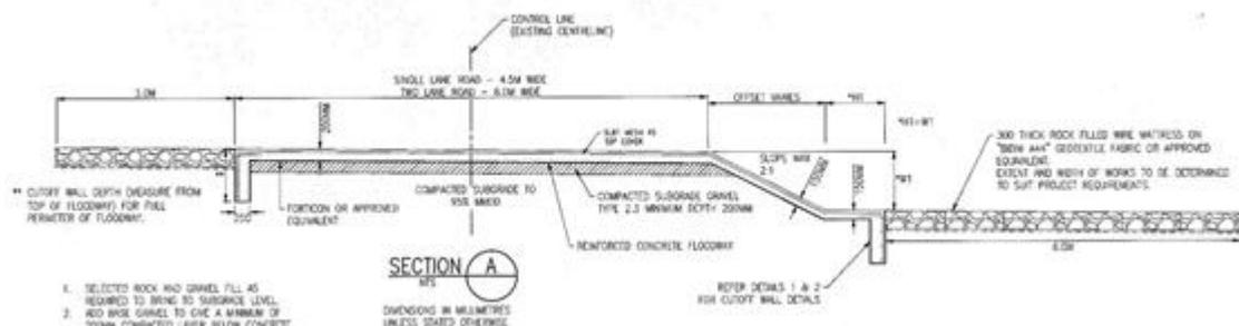
Figure 1 Cross section of floodway Type 2
