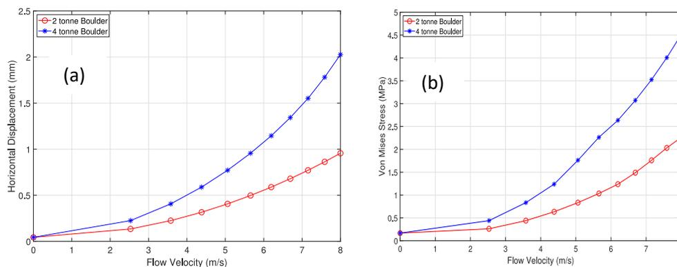
Figure 5 Effect of 2 and 4 tonne boulder impact
