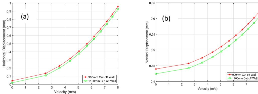
Figure 6 Effect of 2 cut off wall configurations
