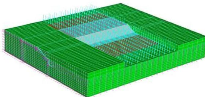
Figure 3 Floodway model with medium mesh size
