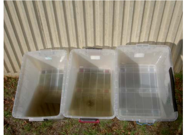
Figure 3 shows samples taken, from left to right, the road, carpark and roof surfaces for a 24mm rainfall event
