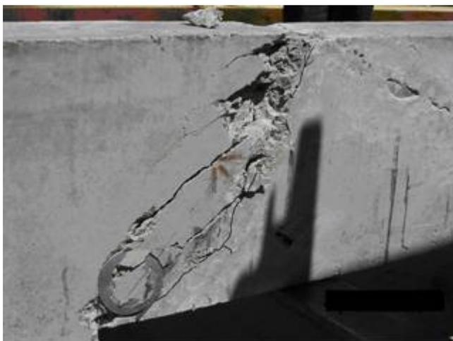
**Fig. 11. Failure of RCH2\* (after epoxy injection)**
