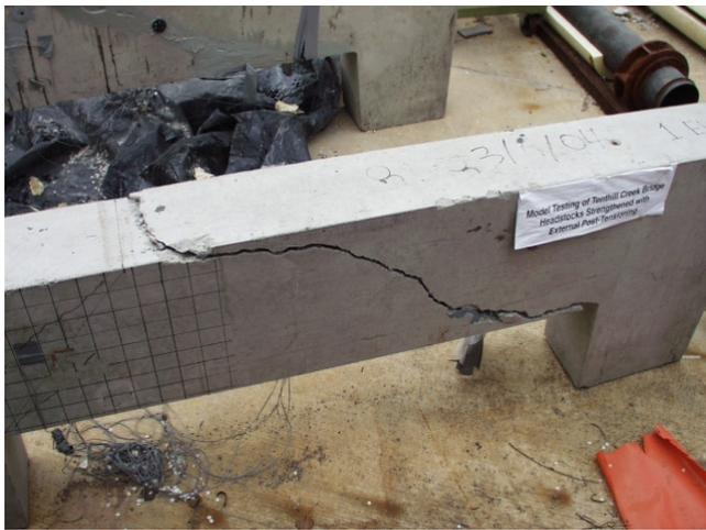
**Fig. 10. Failure of the Control Specimen RCH1**
