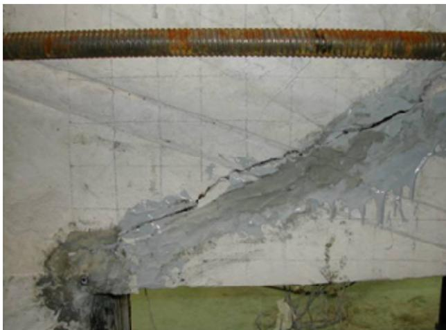
**Fig. 5. New Shear Cracks in RCS3 after Crack Repair**
