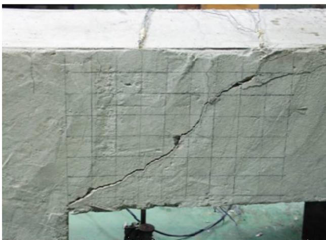
**Fig. 3. Shear Cracks in the Control Specimen RCS1**
