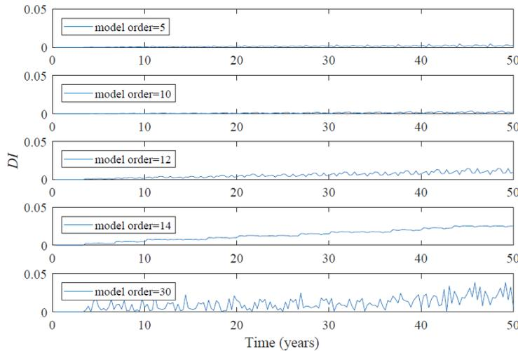
Figure 9. Effect of different model order on  $DI$
