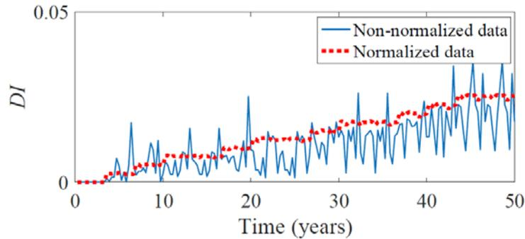
Figure 8. Effect of normalization procedure on  $DI$
