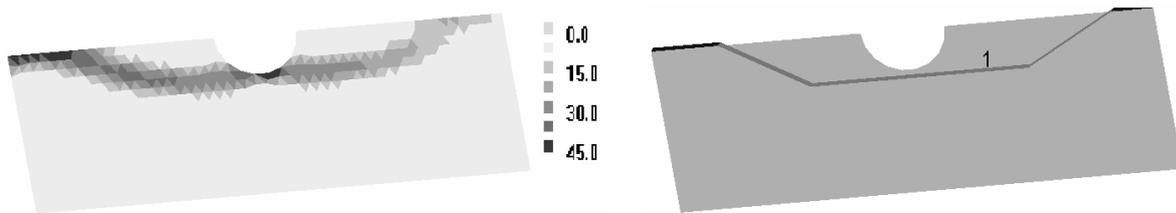
(b) Thickness distribution after stage 1 of optimization process.
