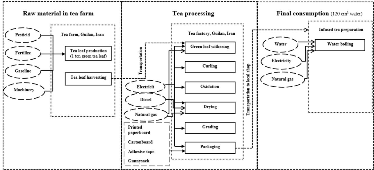
**Fig. 1.** System boundary of tea production cycle (one cup of tea)
