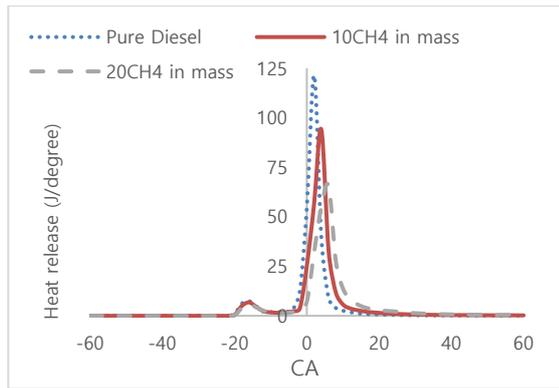
Figure 4: Heat release rate for 2000 rpm.
