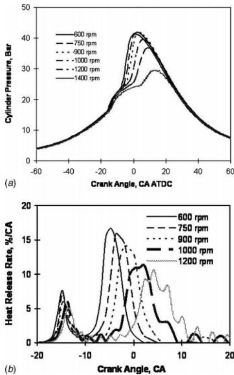
Figure 1: Effect of engine speed on (a) cylinder pressure and (b) heat release rate at CR = 10, AFR = 50,  $T_{in} = 40^\circ\text{C}$  [6].
