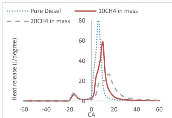
Figure 6: Heat release rate for 2500 rpm.
