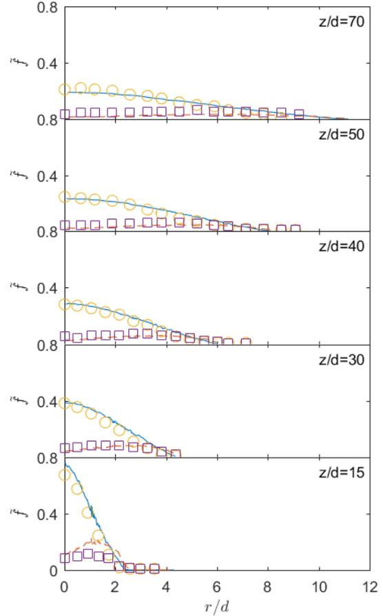
Figure 7: Radial mixture fraction profiles. Mean: MMC, line; expt, circles [14]. rms: MMC, dashed line; expt, squares [14].
