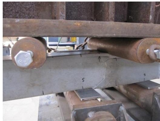
(b) shear test of the beam
