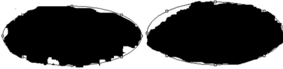
**Figure 6.** Elliptical approximation to weft yarn cross sections for fabric A.
