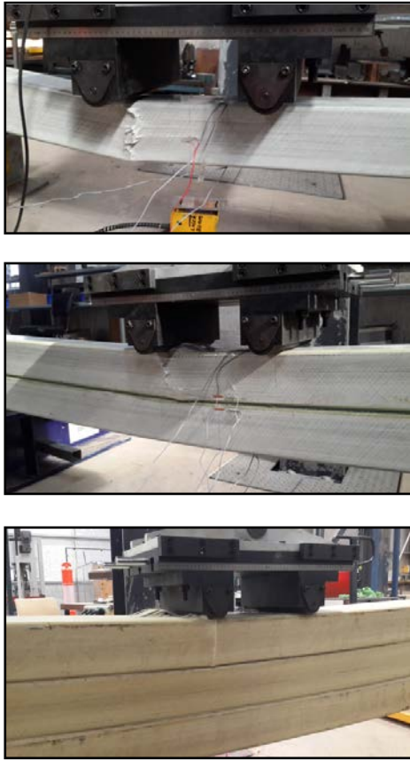
Figure 4. The mode of failure of filled pultruded GFRP beams.
