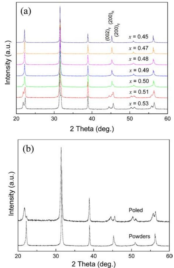
FIG. 1. (a) X-ray diffraction patterns of crushed ceramic powder of  $\text{BMT-}x\text{PT-0.1BZ}$  ( $0.45 \leq x \leq 0.53$ ) at room temperature; (b) x-ray diffraction patterns of crushed ceramic powder and a poled ceramic pellet for the composition of  $\text{BMT-0.48PT-0.1BZ}$ .
