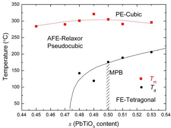
FIG. 8. Phase diagram of BMT- $x$ PT-0.1BZ.
