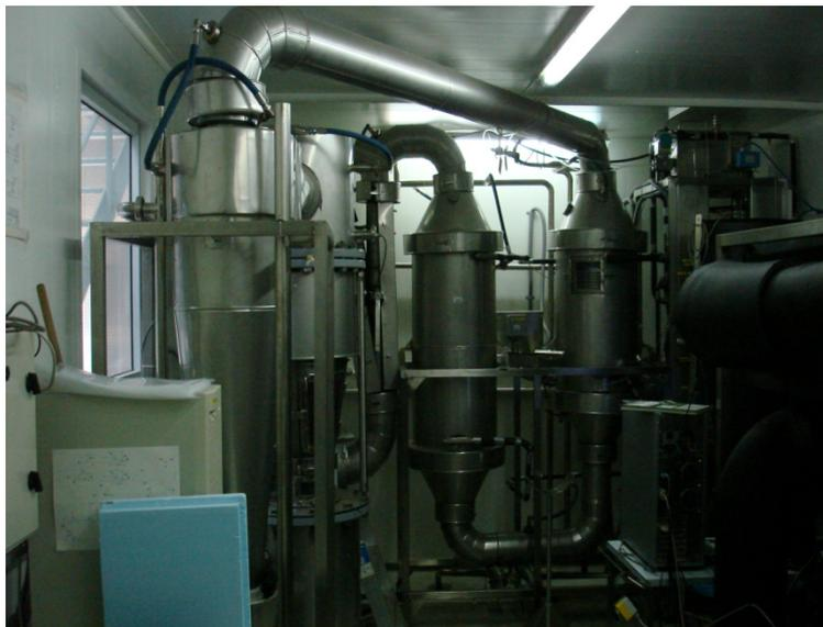
Figure 2. Experimental heat pump fluid bed dryer.
