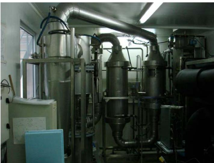
Figure 2. Experimental fluid bed heat pump dryer
