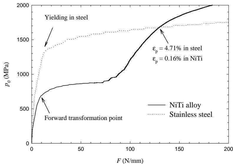
Figure 4. Variation of the maximum contact pressure with the applied contact force from FE simulations for elastic-plastic stainless steel and superelastic-plastic NiTi alloy.
