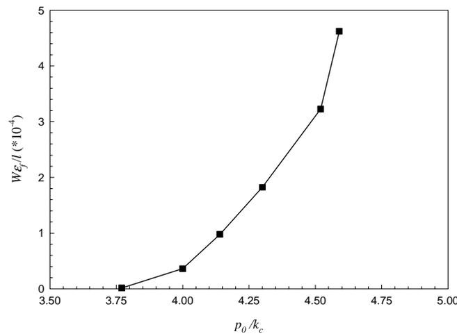
Figure 1. Influence of maximum contact pressure on sliding wear rate.
