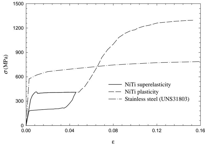
Figure 3. Superelasticity and superelastic-plastic deformation of a NiTi alloy [16] and elastic-plastic deformation of a stainless steel [17].
