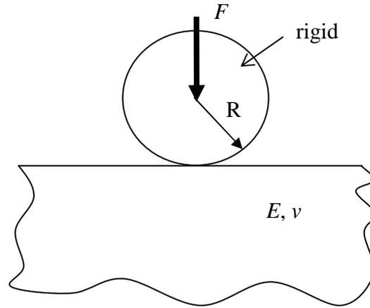
Figure 2. Illustration of a rigid asperity contacting NiTi alloy or steel
