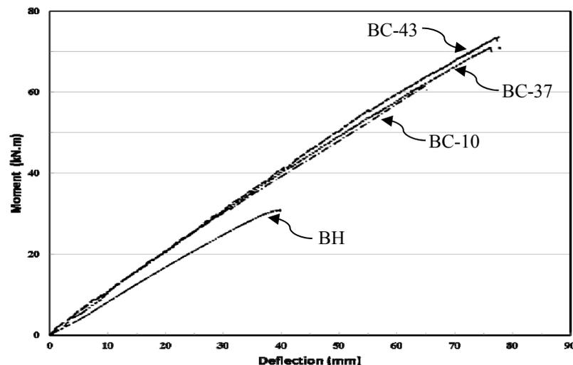
Figure 2 Moment-deflection behaviour of the tested beams.
