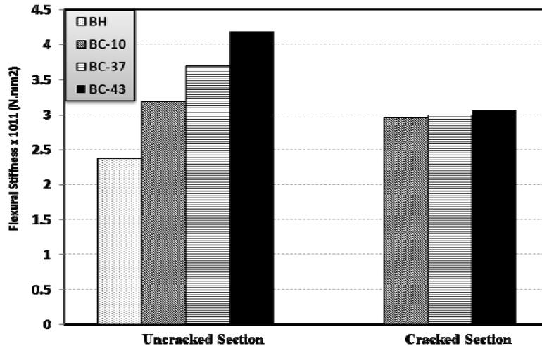
Figure 3 Flexural stiffness of un-cracked and cracked sections.
