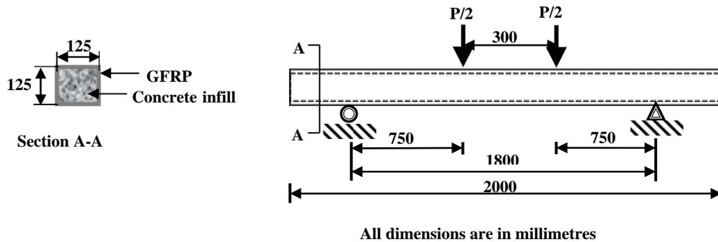
Figure 1 Experimental set up details
