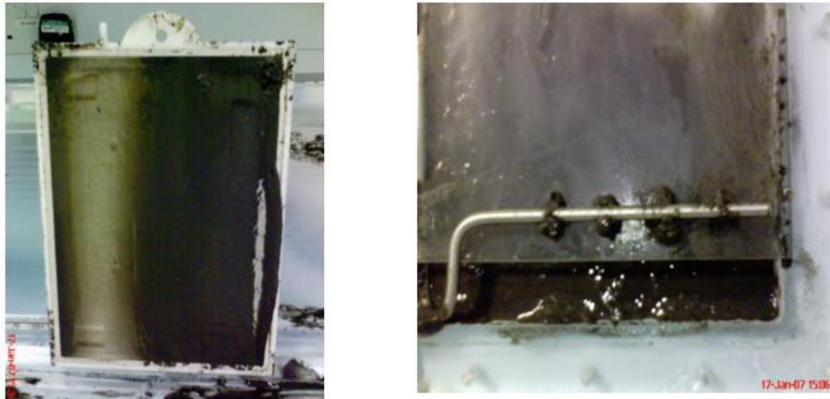
Fig 10. (left) Kubota partially scoured by biogas bubbles. (right) diffuser located at the bottom of the SAMBR with only the far left hole remaining open for gas bubbles formation.
