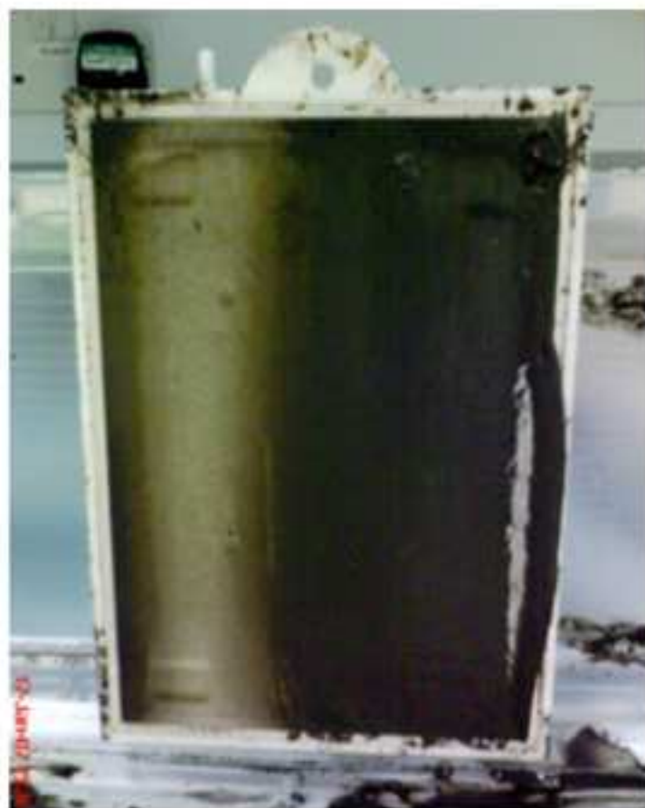
Fig 10. (left) Kubota partially scoured by biogas bubbles. (right) diffuser located at the bottom of the SAMBR with only the far left hole remaining open for gas bubbles formation.
