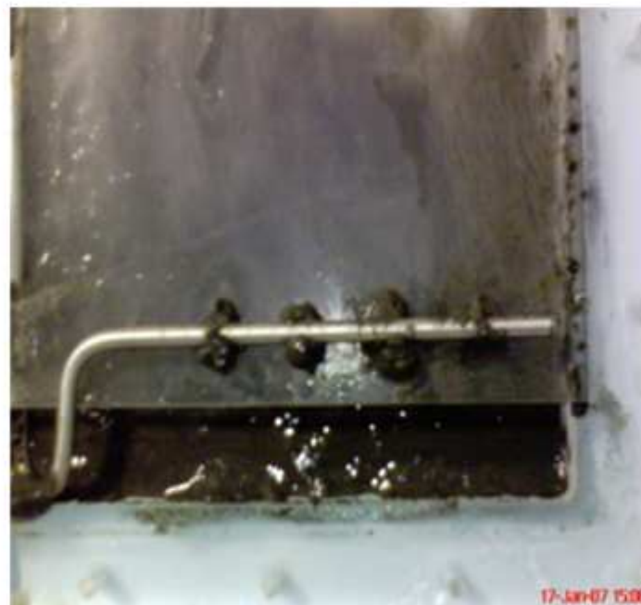
Fig 10. (left) Kubota partially scoured by biogas bubbles. (right) diffuser located at the bottom of the SAMBR with only the far left hole remaining open for gas bubbles formation.
