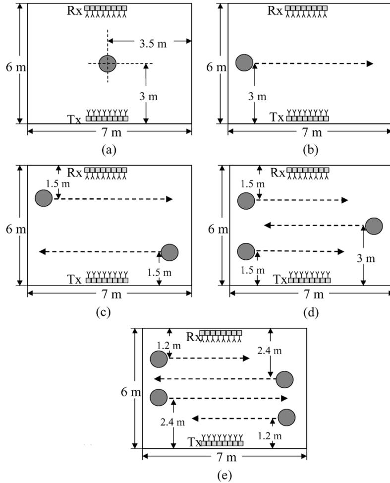
Fig. 4. Simulated scenarios (top view) for the pedestrian trajectories given in Table II. (a) 1NLOS. (b) 1A. (c) 2A and 2B. (d) 3A and 3B. (e) 4A and 4B.
