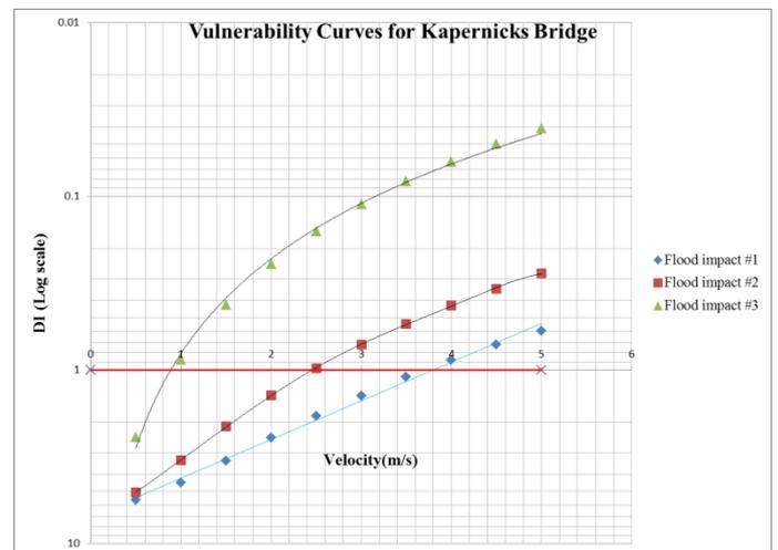
Fig 4: Vulnerability curves for Kapernicks Bridge
