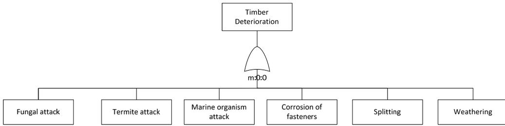
Figure 4: Major sub system fault tree of timber deterioration
