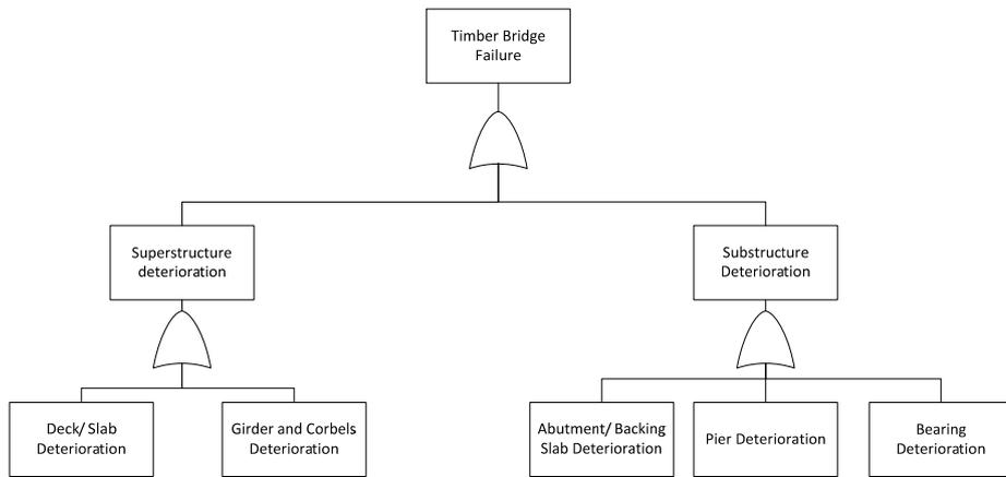
Figure 3: Top level fault tree frame
