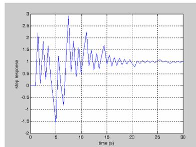
Fig. 5 Overall Step Response of the System
