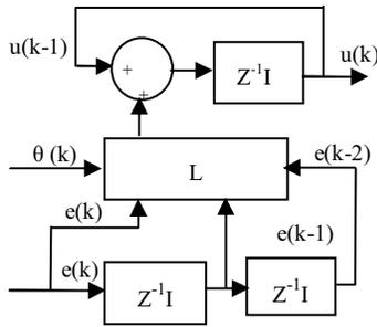
Fig. 2 PID Controller over NCS with Markov Chain
