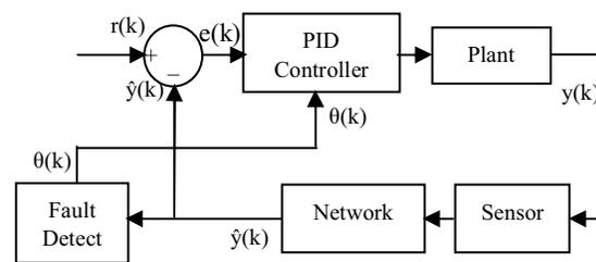
Fig. 1 Networked Control System with PID Controller
