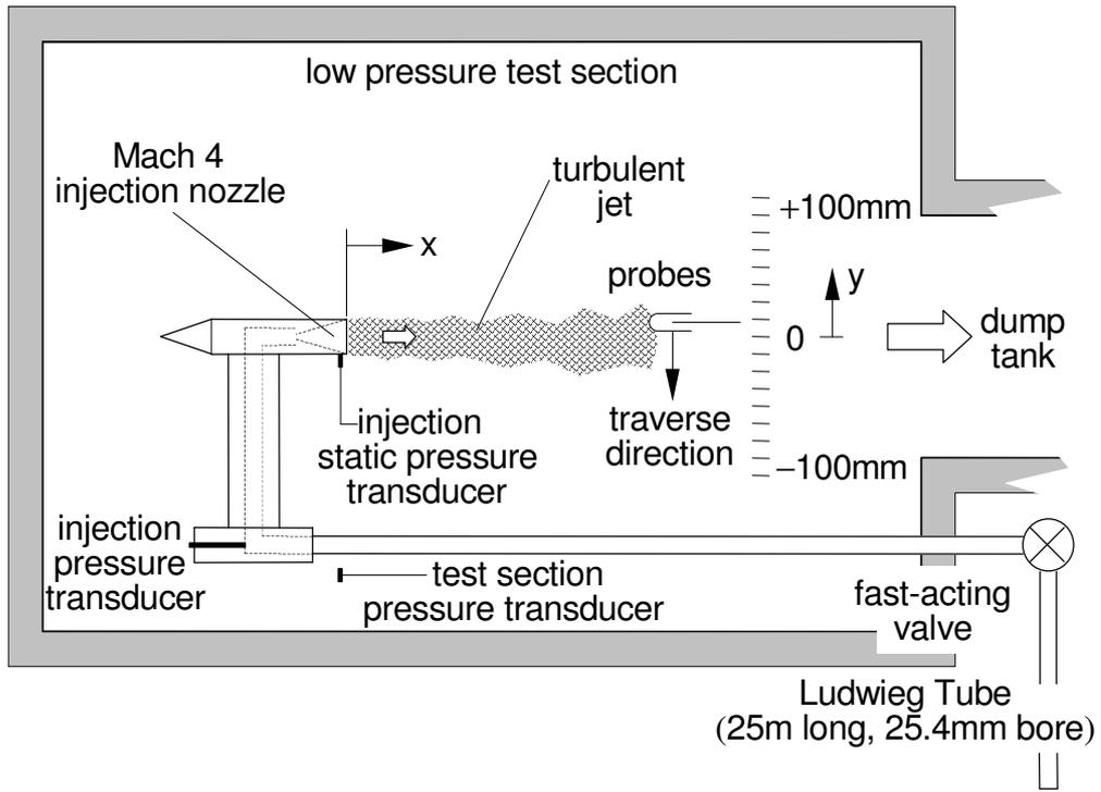
**Fig. 3.** Illustration of the Mach 4 free jet arrangement
