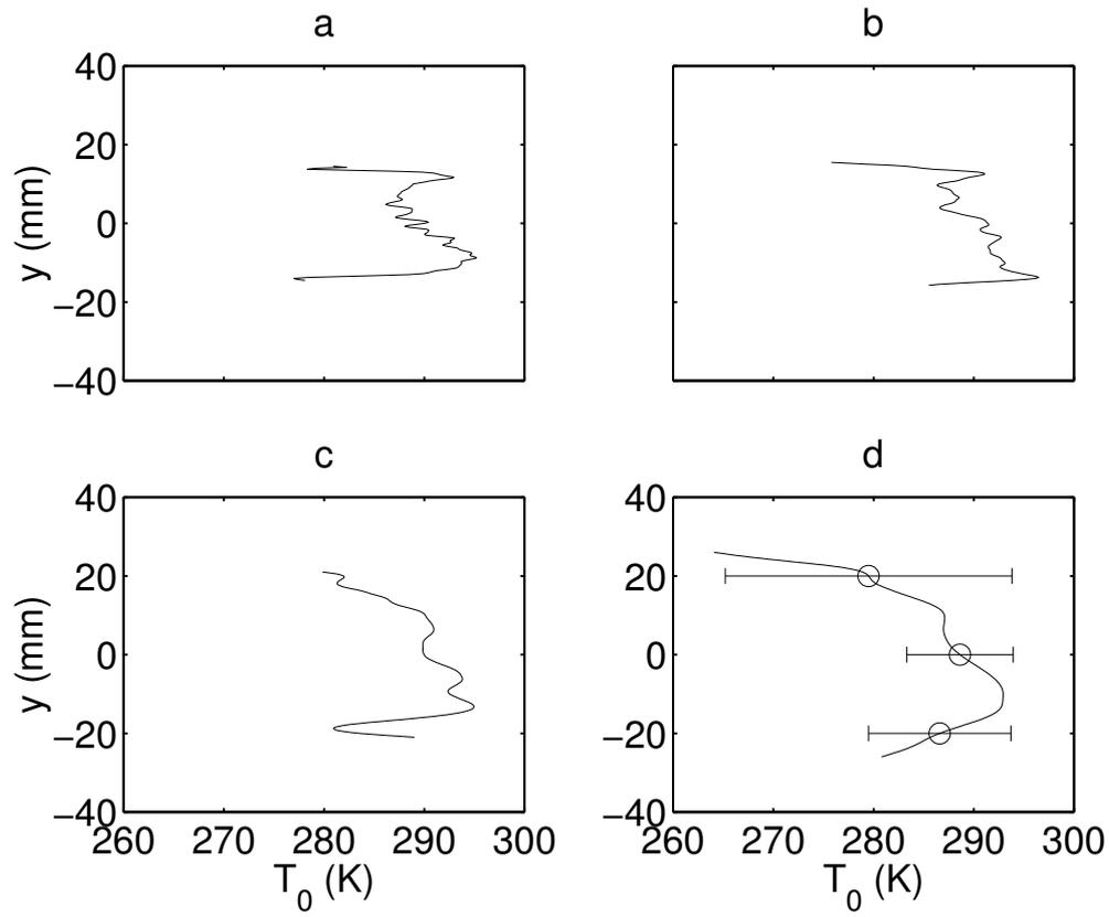
**Fig. 6a-d.** Time-averaged stagnation temperature measurements at 4 stations downstream of injection.
