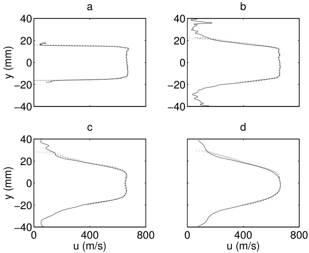
**Fig. 9a-d.** Time-averaged velocity profiles at 4 stations downstream of injection. **a**  $x=1$  mm; **b**  $x=100$  mm; **c**  $x=200$  mm; **d**  $x=300$  mm. Solid line: derived from heat transfer coefficient measurements; dots: derived from pitot pressure measurements
