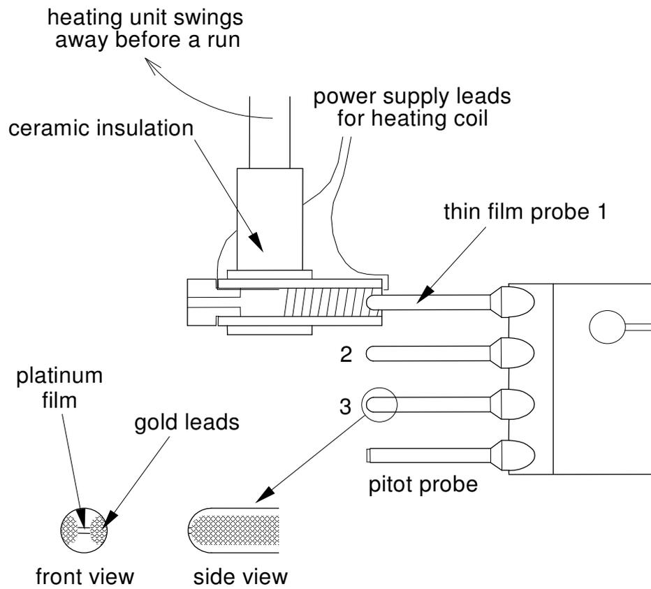
**Fig.1.** Illustration of the probe arrangement
