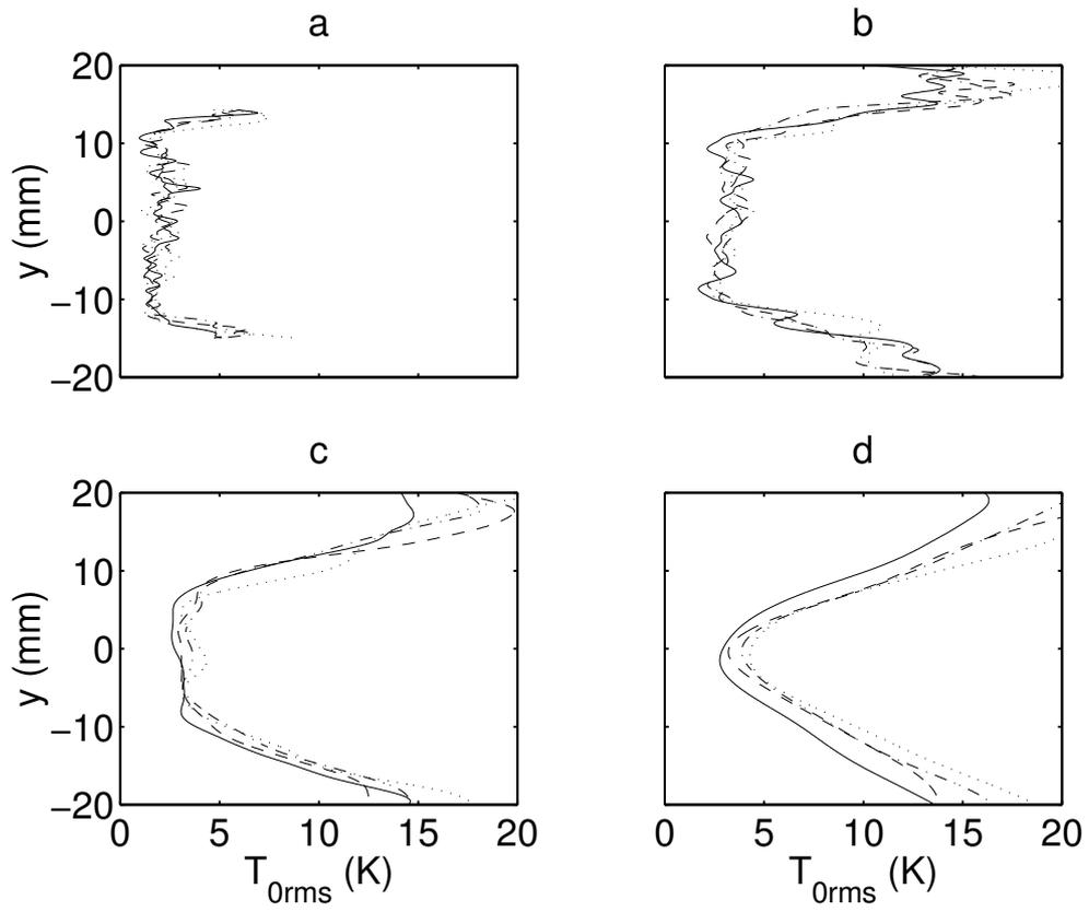
**Fig. 10a-d.** RMS stagnation temperature fluctuations at 4 stations downstream of injection. **a**  $x=1$  mm; **b**  $x=100$  mm; **c**  $x=200$  mm; **d**  $x=300$  mm. Solid line:  $\overline{T_0} - \overline{T_w} \approx -25$  K; dots:  $\overline{T_0} - \overline{T_w} \approx -60$  K; other lines: intermediate temperatures
