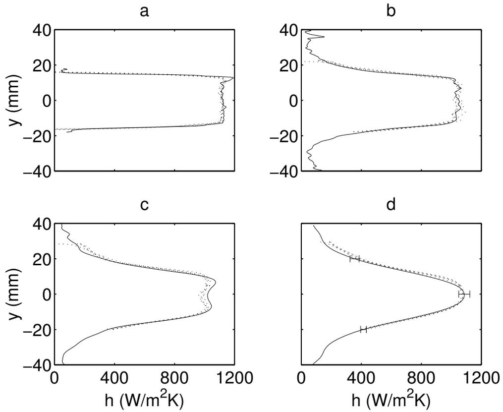
**Fig. 7a-d.** Time-averaged heat transfer coefficient results at 4 stations downstream of injection. **a**  $x=1$  mm; **b**  $x=100$  mm; **c**  $x=200$  mm; **d**  $x=300$  mm. Solid line: thin film heat transfer coefficient measurements; dots: derived from pitot pressure measurements
