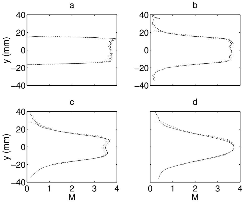
**Fig. 8a-d.** Time-averaged Mach number profiles at 4 stations downstream of injection. **a**  $x=1$  mm; **b**  $x=100$  mm; **c**  $x=200$  mm; **d**  $x=300$  mm. Solid line: derived from heat transfer coefficient measurements; dots: derived from pitot pressure measurements
