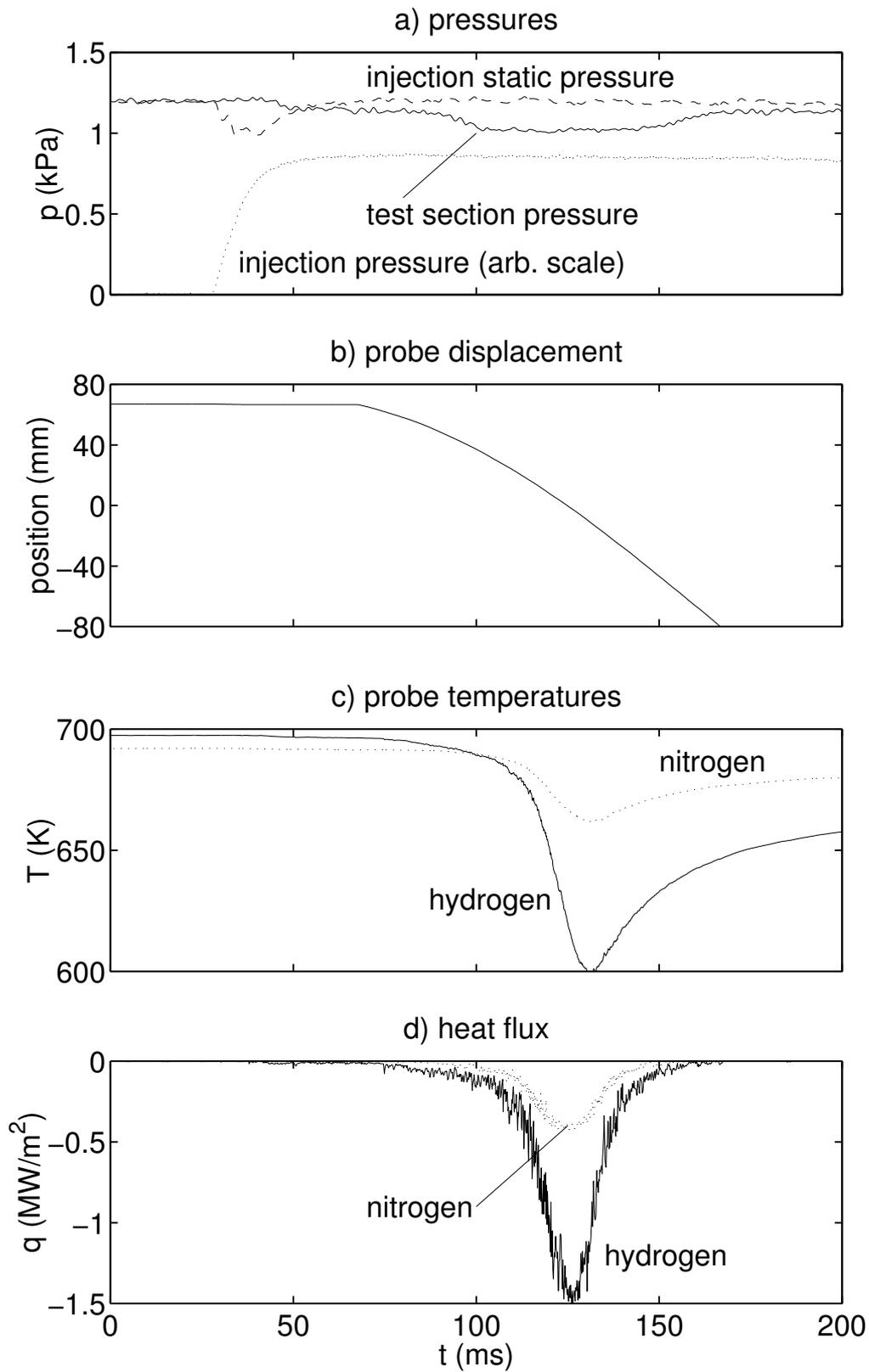
**Fig. 5 Typical signals obtained during the experiments**
