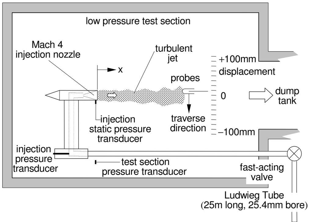
**Fig. 4 Illustration of the Mach 4 free jet arrangement**
