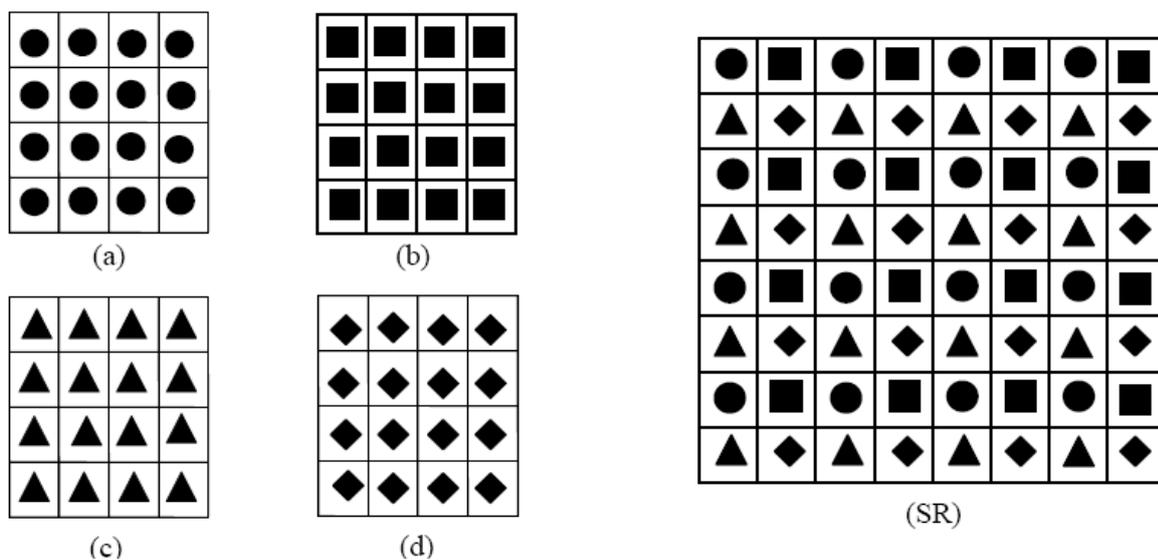
Figure 1 - An idealized super-resolution setup. Images (b)-(d) are taken with sub-pixel shifts of half a pixel in the horizontal, vertical and diagonal directions in relation to image (a). Their pixels can then be interleaved to generate a double resolution image in each coordinate direction.
