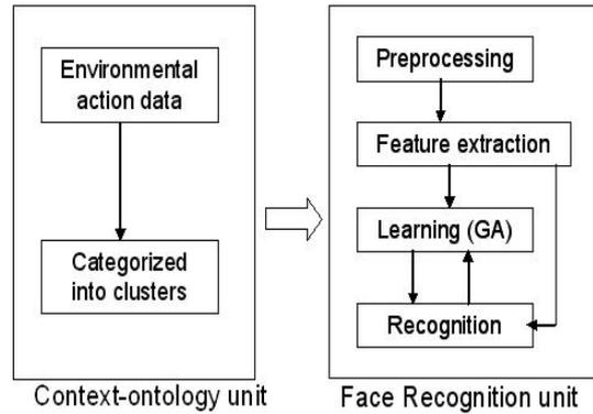
Fig 4. Block diagram of proposed context ontology based face recognition
