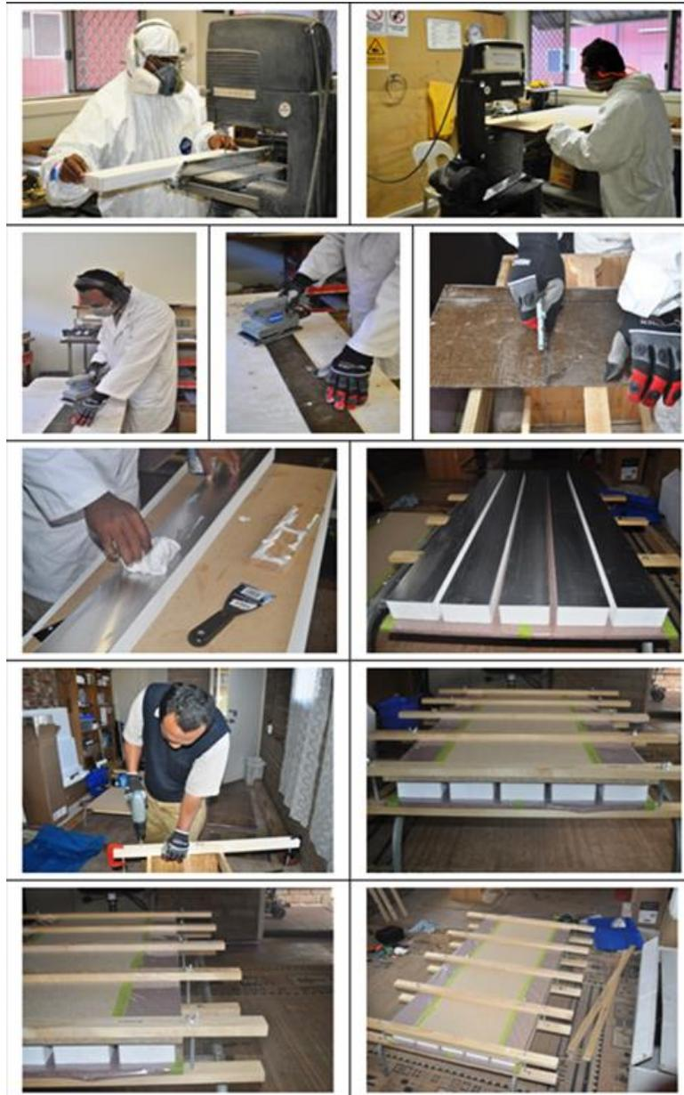
Figure 3 Sandwich panel fabrication process
