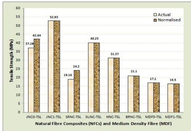
Figure 2 Tensile strength of NFCs and MDF
