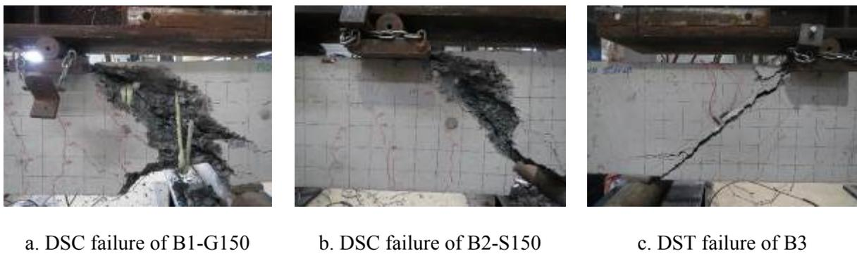
Figure 5 Failure mode of the tested beams.
