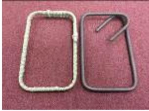
Figure 1 GFRP and steel stirrups.
