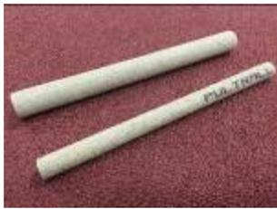
Figure 2 Sand-coated GFRP bars.
