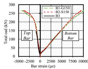
Figure 7 Shear load-longitudinal bar strain relationship.
