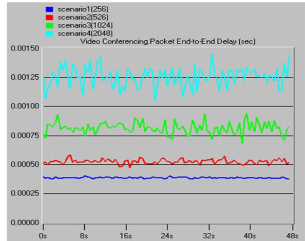
Fig. 6. Comparison of end-to-end *transmission delay* messages in different packet sizes.
