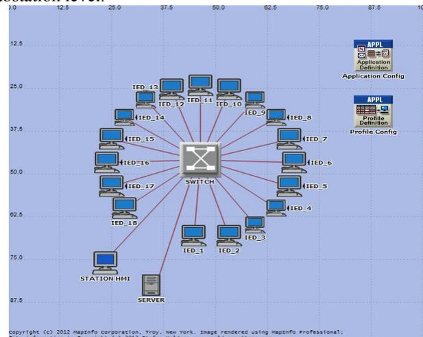
Fig. 4. Station level network simulation model by OPNET.
