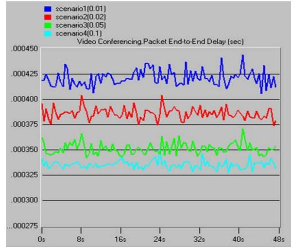
Fig. 5. Comparison of end-to-end *transmission delay* messages in different packet interval.
