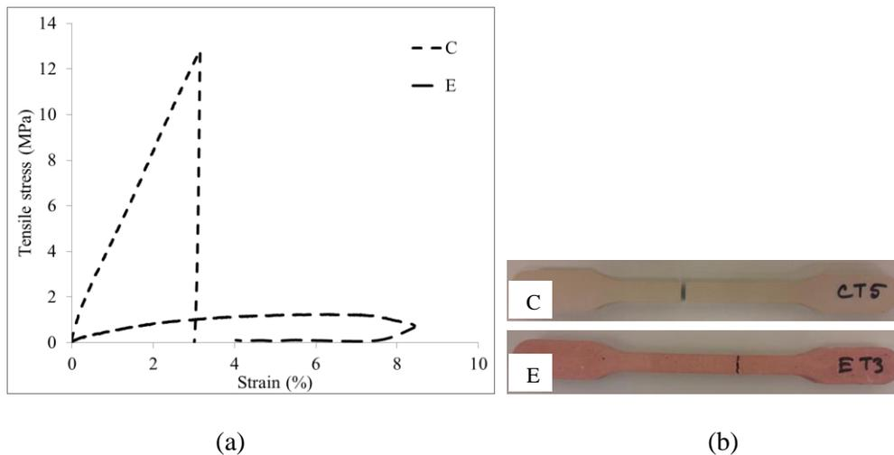
Figure 3. Typical tensile behavior; (a) stress-strain, and (b) failure pattern of the specimens
