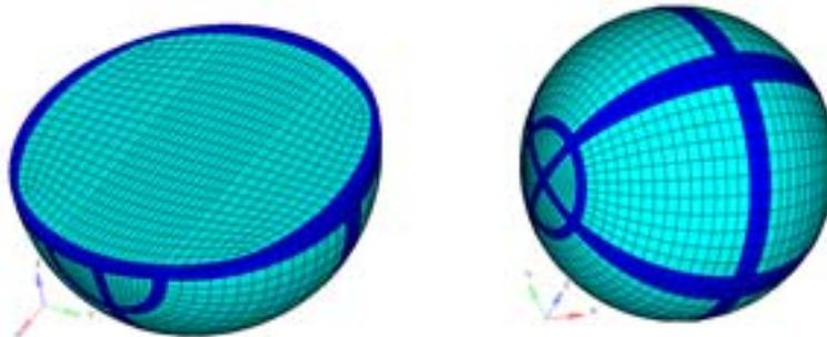
**Figure 2:** Finite Element model of the baseball
